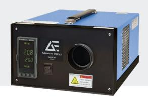
The Mikron® M340 is a portable blackbody calibration source covering the range from sub-zero to 150°C with 0.1° resolution. The thermoelectric heating/cooling mechanism is utilized to achieve a compact and easy-to-use blackbody source. The M340 has unusually high temperature stability and a stabilization time of only 10 minutes. Source temperature is closely controlled by a self-tuning PID controller which displays temperature on a digital readout.
