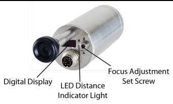
The LED Distance Indicator Light (labeled mm) will turn red and the approximate focused measuring distance in mm will automatically be shown on the Digital Display for a few seconds after making an adjustment using the Focus Adjustment Set Screw.
